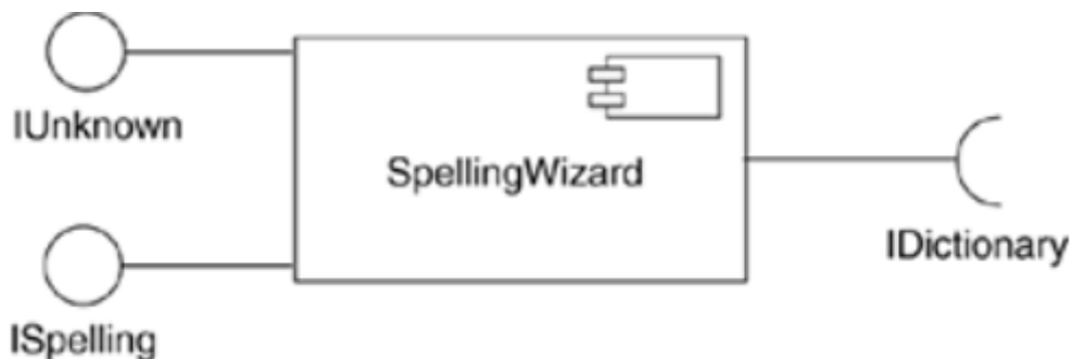
Figure 25. Example of division by separating interface from implementation
