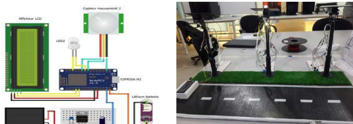
Figure I. 9 - Simplified schematic of the intelligent urban lighting system and the developed prototype.
