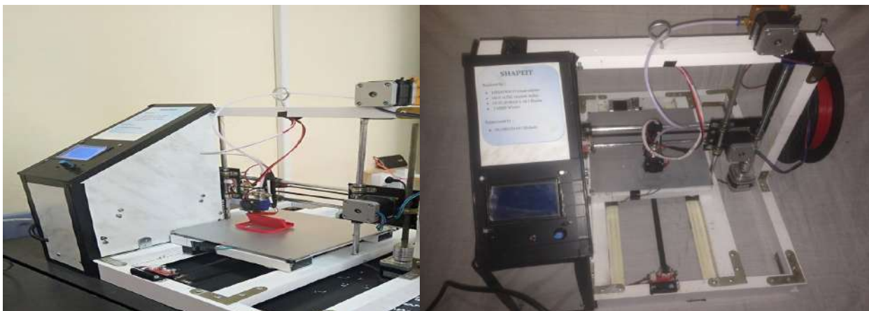
Figure I. 7 - Prototype of the 3D printer (Version 1) developed by engineering students, showing the mechanical frame, control electronics, and software interface.
